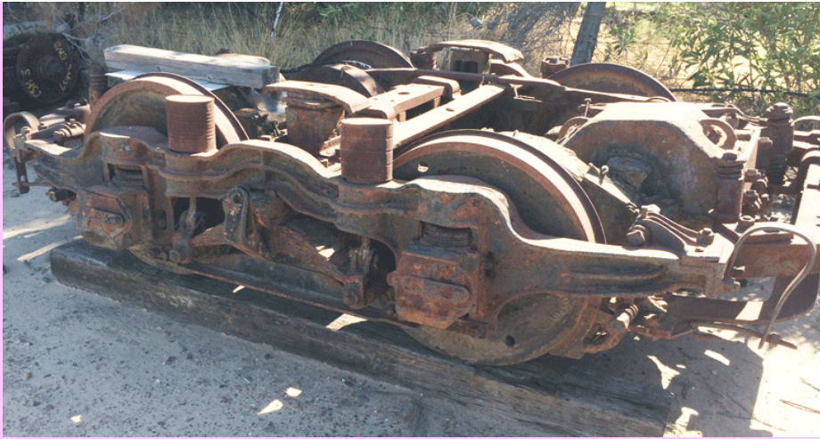
The above truck appears to be a Peckham 14-B-3-S as was used in San Francisco, California.
